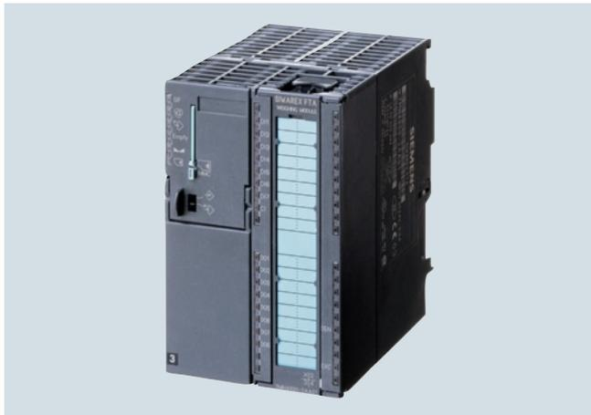
The SIWAREX FTA (Flexible Technology, Automatic Weighing Instrument) is a versatile and flexible weighing module for industrial use. It can be used in both non-automatic and automatic weighing operation, for example the production of mixtures, and for filling, loading, monitoring and bag filling.
